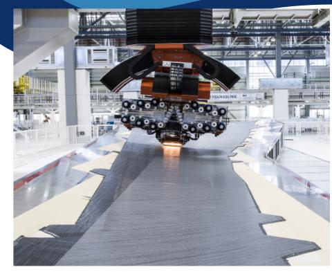
Automated Fiber Placement (AFP) and Automated Tape Layup (ATL) are methods to fabricate near-net-shape fiber-reinforced parts using a CNC machine to apply layers of material to a mold.
