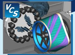
Reads CAD geometry of the layup form, machine axes, and work cell
