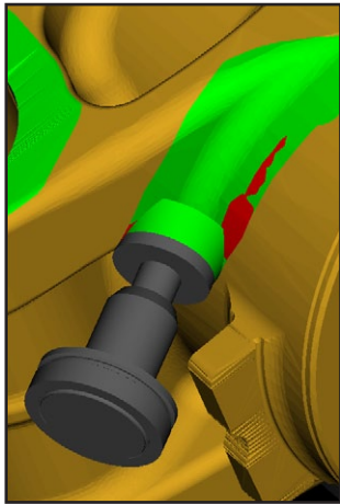
A new "Polishing Tool" uses two shapes to represent a polishing region, with an inside and outside limit. Color is applied to the stock surface by intersecting with the polishing tool. If the inside limit comes in contact with the cut stock, an error is created.
