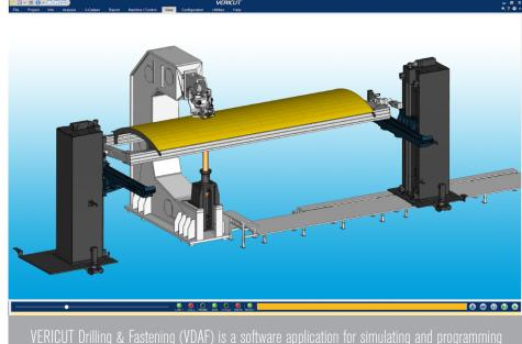
'ERICUT Drilling & Fastening (VDAF) is a software application for simulating and programming uto-drilling & fastening machines. VDAF is independent of both the machine and CAD system
