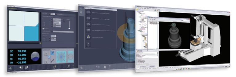
Use the ZOLLER vision system software to scan the physical tool on the presetter then utilize the scanned geometry in VERI-CUT for a CNC simulation. ZOLLER vision system software is fully automatic and precise to the micron. A DXF file is created from scanning the tool showing the exact shape of the assembly geometry. This data can then be stored within ZOLLER TMS and also accessed by VERICUT.
