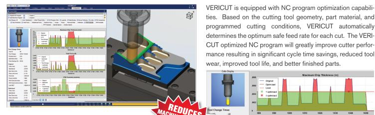
programmed cutting conditions, VERICUT automatically determines the optimum safe feed rate for each cut. The VERI-CUT optimized NC program will greatly improve cutter performance resulting in significant cycle time savings, reduced tool wear, improved tool life, and better finished parts.
