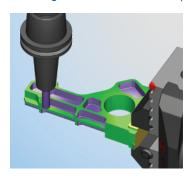
VERICUT simulates milling, drilling, turning, multi-tasking mill/turn, and EDM operations. Errors that could ruin the part, damage the fixture, or break the cutting tool are easily identified. VERICUT supports G-codes and native CAM files and includes analysis tools to measure and compare the cut part with the design model. You can model any cutter, fixture, or holder shape. During simulation you create in-process inspection instructions and export a CAD model of the "as-machined" part.
