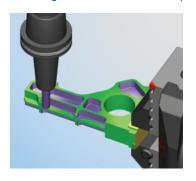
VERICUT simulates milling, drilling, turning, multi-tasking mill/turn, and EDM operations. Errors that could ruin the part, damage the fixture, or break the cutting tool are easily identified. VERICUT supports G-codes and native CAM files and includes analysis tools to measure and compare the cut part with the design model. You can model any cutter, fixture, or holder shape. During simulation you create in-process inspection instructions and export a CAD model of the "as-machined" part.
