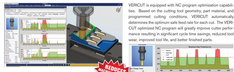
programmed cutting conditions, VERICUT automatically determines the optimum safe feed rate for each cut. The VERI-CUT optimized NC program will greatly improve cutter performance resulting in significant cycle time savings, reduced tool wear, improved tool life, and better finished parts.
