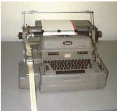
A Flexowriter machine was needed to type paper tape code used to guide the movements of an NC cutting machine.
