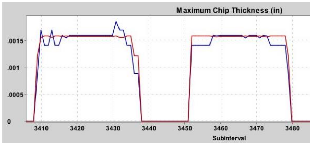
Figure 9 - Optimization of a 1/2" Endmill in red, the shock of the tool from the original code has been eliminated
