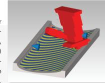
VCP reads CAD surfaces and ply boundary information and adds material to fill the plies according to user-specified manufacturing standards and requirements. Layup paths are then linked together to form specific layup sequences and output as
